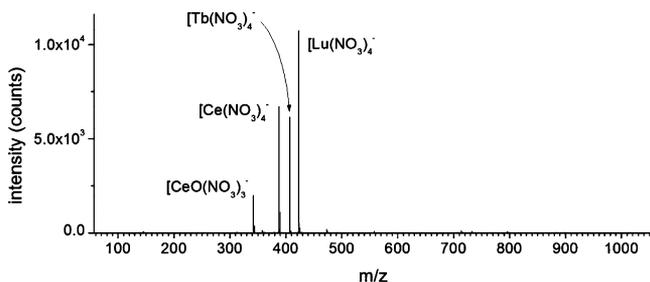
**Figure 1.** Negative ion mass spectrum of a single 17 nL droplet of a lanthanide nitrate solution (293  $\mu\text{M}$ ).
