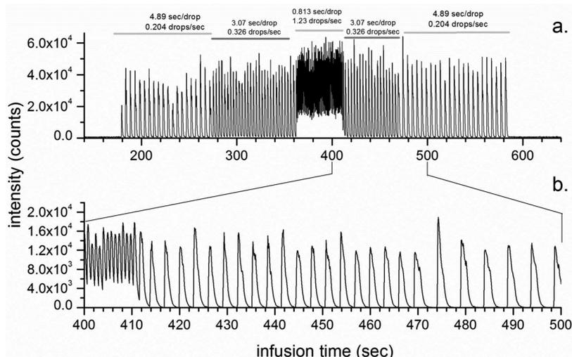
**Figure 3.** Infusion profiles of a series of individual droplets. (a) Total ion profile, showing five different frequency regimes. (b) Extracted ion profile of  $m/z$  422.9,  $[\text{Lu}(\text{NO}_3)_4]^-$  from 400 to 500 s.
