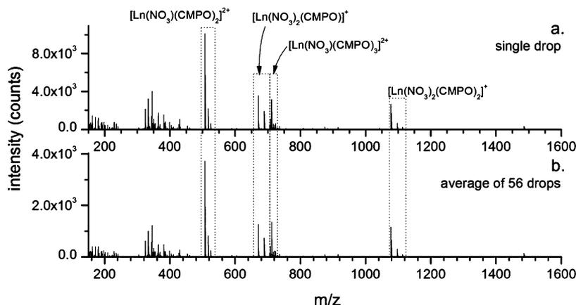
**Figure 5.** Positive ion spectra of a solution of Ce, Tb, and Lu nitrates with CMPO.
