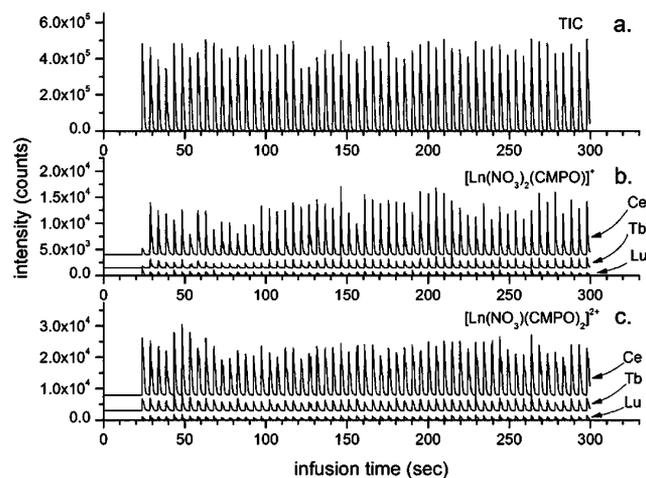
**Figure 7.** Positive ion profiles generated by individual drops. (a) Total ion current. (b) Singly charged complexes, [Ln(NO<sub>3</sub>)<sub>2</sub>(CMPO)]<sup>+</sup>. (c) Doubly charged complexes, [Ln(NO<sub>3</sub>)(CMPO)<sub>2</sub>]<sup>2+</sup>. The Ce and Tb profiles are offset from the baseline.
