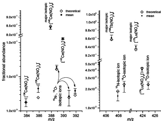
**Figure 2.** Comparison of abundances of minor isotopes with theoretical values. Left,  $[\text{Ce}(\text{NO}_3)_4]^-$  isotopic ions. Right,  $[\text{Tb}(\text{NO}_3)_4]^-$  and  $[\text{Lu}(\text{NO}_3)_4]^-$  isotopic ions. Filled circles are averages of five droplets, with one standard deviation error bar. Open diamonds are theoretical values for the isotopic ions.
