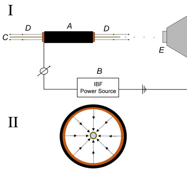
**Figure 1.** Schematic of inductor employed in this work, inspired by R.W. Kiser<sup>2</sup>
