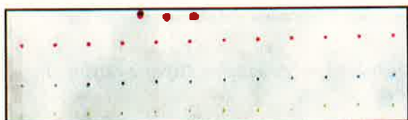
Figure 6 Three liquids dispensed at three different rates from three different radii, 7 sec per tridispense. Mean values estimated as discussed previously: green, 71 nL, blue, 143 nL; and red, 189 nL, with CVs of 25.6, 19.4, and 11.8% respectively. Note: The source of error involves the entire process of dispensing, drying, and software/data analysis.
