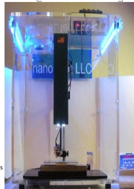
Parallel dispense, 384 channels, in 1 ms!
